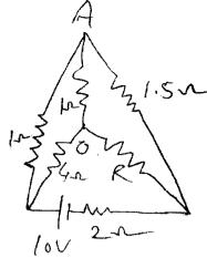
f. Using mesh analysis find the branch current in following network:
